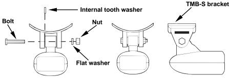
Attach motor mounting bracket to transducer.
